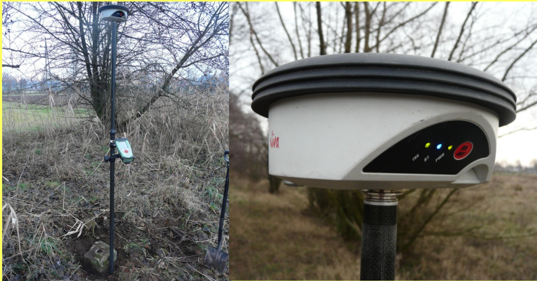
Rys. 14. Leica Viva NetRover, kontroler CS10, antena GS08.
